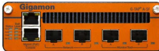
The G-TAP A-SF accepts SFP and SFP+ transceivers as well as Direct Attach Cables for the Network and Monitor/Tool ports. The transceivers in the **Network A and B** ports must match for successful traffic flow (for example, two SFP SR transceivers).
