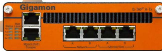
Serial Console port accepts terminal connections for configuration of G-TAP A Series settings, including time, network, and SNMP settings. Speed is configurable in CLI – default settings are 8N1, 115,200 bps.
