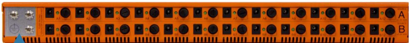
The chassis ground screws are at the rear of the unit. Connect grounding wire here and to earth ground.
